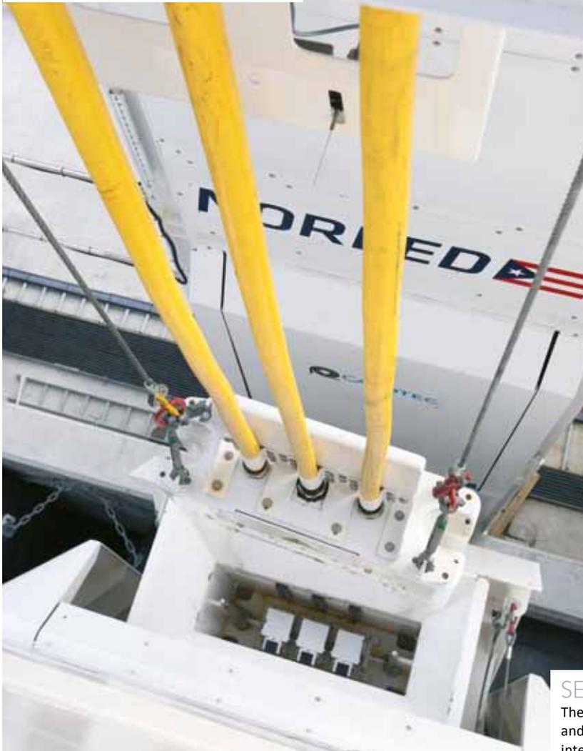
The Ampere was developed from the ground up as an electrically powered vessel, made exclusively of aluminum. With three battery packs, one on board and one at each pier, the ferry only uses 150kWh per route, which corresponds to three days use of electricity in a standard Norwegian household. Siemens developed the ferry's drive system and put up charging stations with lithium-ion batteries, which are charged from renewable energy, namely hydro power.
